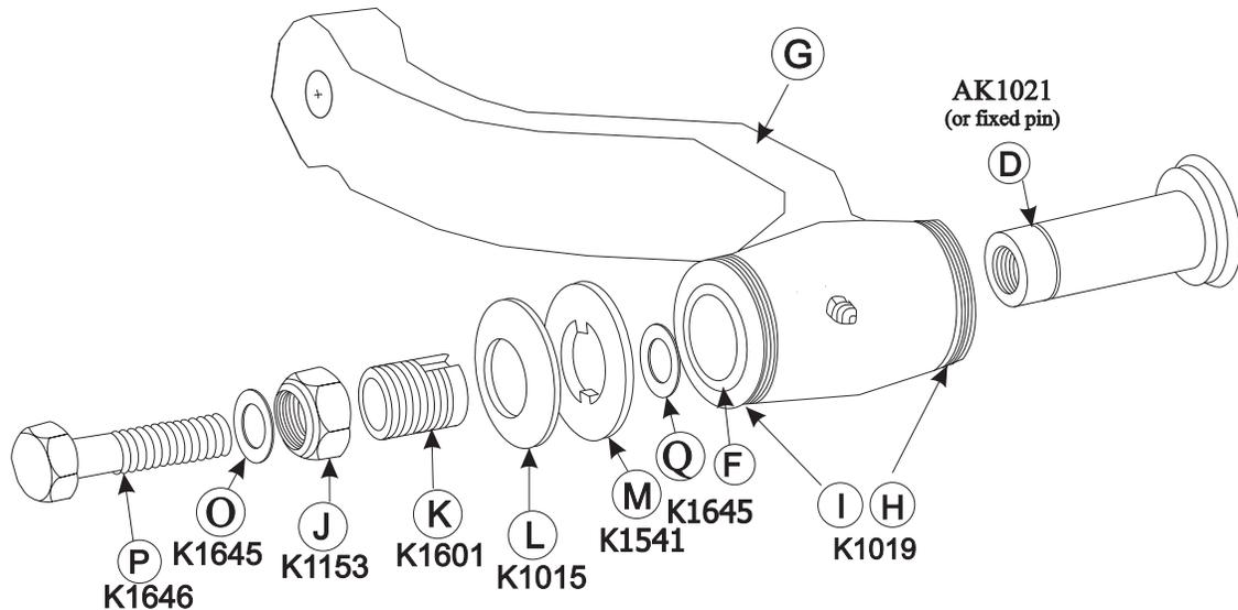
9. Tighten locknut (J) to increase the disc spring pressure on the hub of the arm to the point that when the wheel is raised it will just stay up. It should take a small force to push the wheel down. Do not over-tighten.
