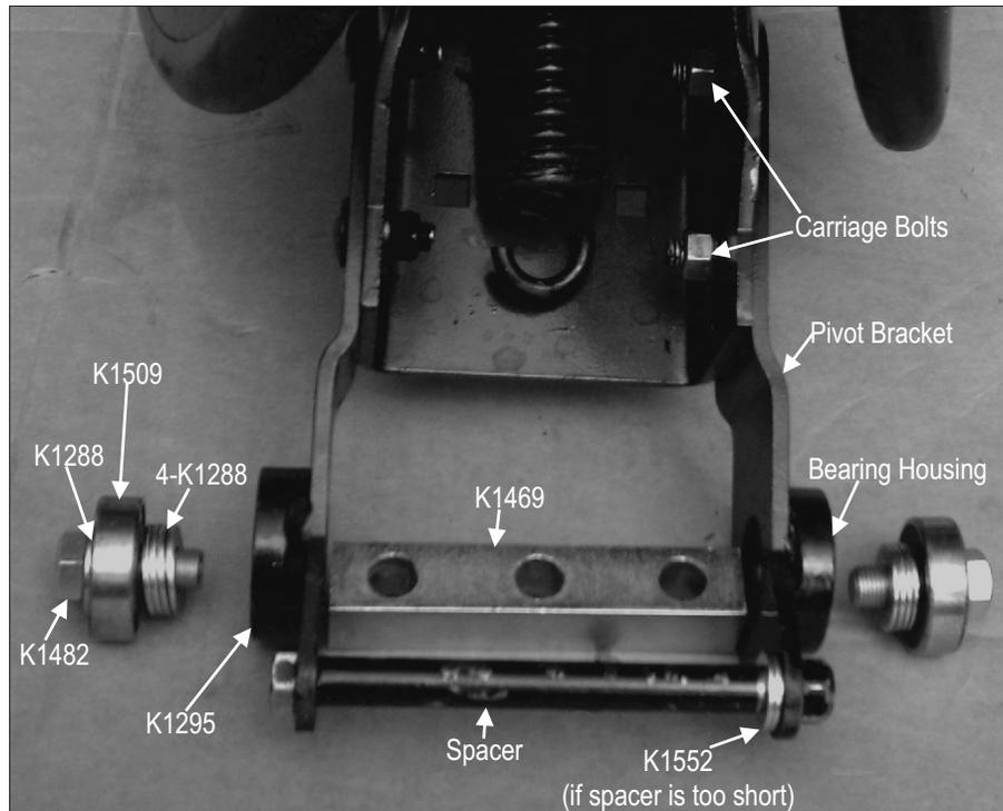
1. Position bearing housings concentric with original holes. Clamp housings to pivot brackets and weld with a 1" weld top and bottom.
