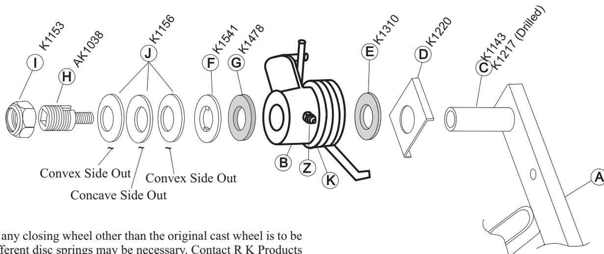
Note: If any closing wheel other than the original cast wheel is to be used different disc springs may be necessary. Contact R K Products for information.
